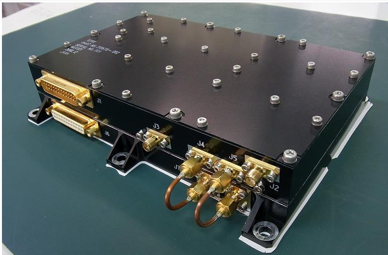
Upper section : USB transceiver unit
