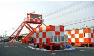
Right: Power Supply Shelter Center: Communication Shelter Back: Control Shelter and Lifter
