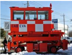
Control Shelter Lowered by Lifter
