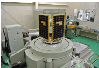
SmallSat "TSUBAME" Located on the Bench of Vibration Test Equipment
