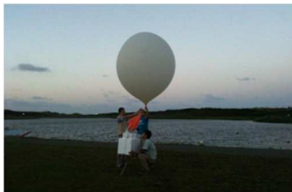
A Scene of CO2 Radiosonde Deployment in Hokkaido Teshio Town
