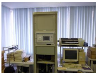
Seismic Intensity Alert System Installed in the Control Office of Suno Dam
