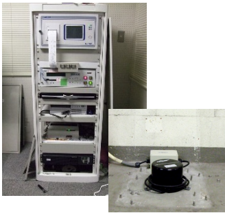
Seismic Intensity System and Seismic Intensity Meter (lower right)
