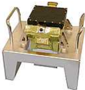
Fluorescent X-Ray Spectrometer on the "HAYABUSA"
