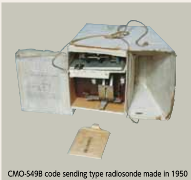
CMO-S48B code sending type radiosonde made in 1950
