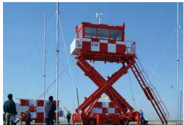
Control tower system with an elevating module
