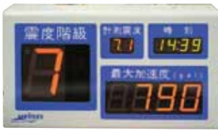
Display unit of the seismic intensity meter
