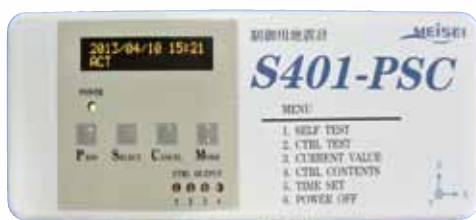
External system control seismometer
